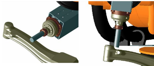
Figure 2. Left: Machining with the tool lateral. Right: Machining with the tool frontal.
